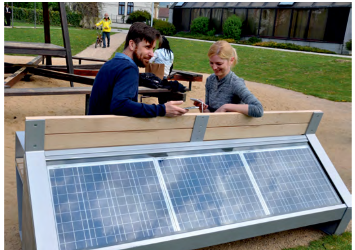
FullCapacity solar bench with a Wi-Fi hotspot and charging sockets. The City of Litoměřice, Czech Republic (Source: The City of Litoměřice)
